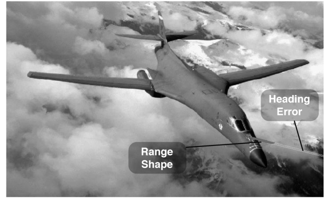
Fig. 10 Illustration of range shape and heading errors, visual position sensing simulation.
