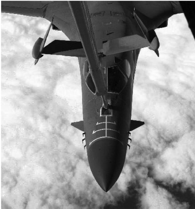
Fig. 2 B-1B Lancer refueling from a KC-135 using boom and receptacle method.
